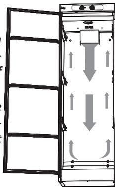
**Note:** When the cabinet is cold it may happen that the door's sealing strip does not close completely. However, this is fully compensated when the cabinet is operating with heat as the sealing strip expands.
