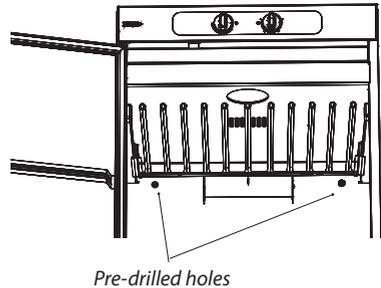
*Attaching to a wall also means a better door seal.*
