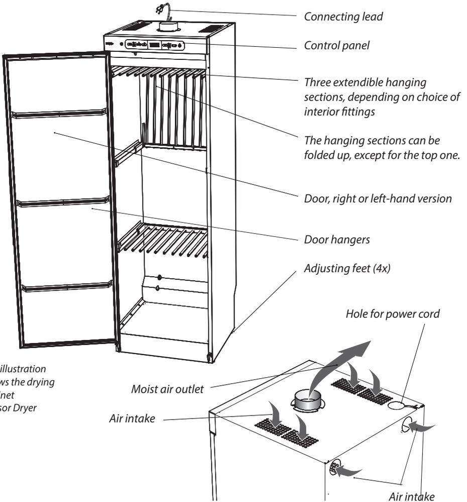
The illustration shows the drying cabinet Sensor Dryer
