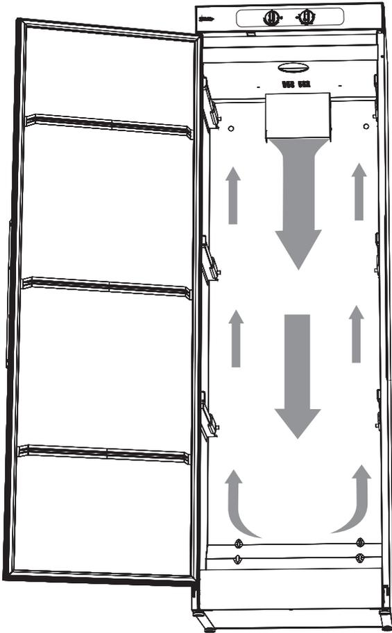
Note the direction of air flow inside the cabinet when positioning laundry. See also this section.
