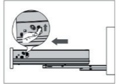
Lift the release handle and pull out the drawer.
